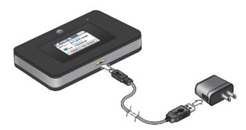
Connect the other end of the cable to the USB port on your computer or to the USB charger.
