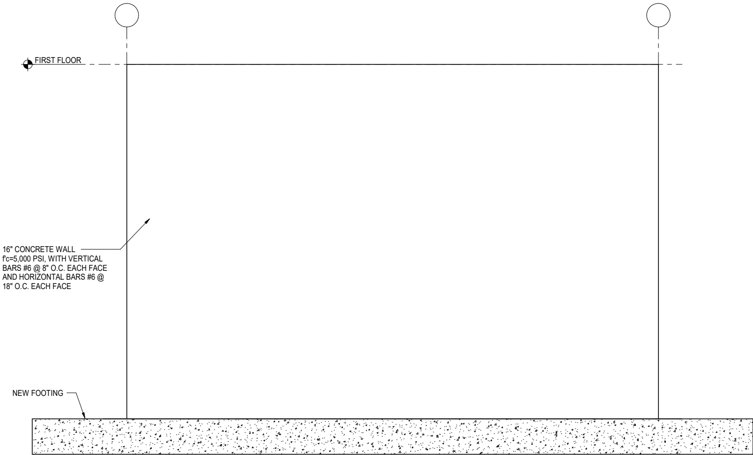
1 TYPICAL CONCRETE SHEAR WALL ELEVATION
